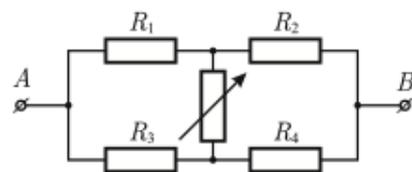
$$R_3 = \frac{R_1 R_4}{R_2} = 40 \text{ Ом}; R_{AB} = \frac{(R_1 + R_2)(R_3 + R_4)}{R_1 + R_2 + R_3 + R_4} \approx 33 \text{ Ом}$$
