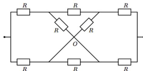
$$\boxed{\text{а) } R_{AB} = \frac{5}{6}R; \text{ б) } R_{AB} = \frac{7}{8}R}$$
