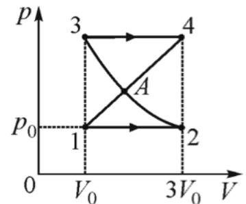
$$Q_{14} = \int_{V_0}^{3V_0} p dV = \int_{V_0}^{3V_0} \left( \frac{p_0 V_0}{V} + \frac{p_0 V_0}{3V_0 - V} \right) dV = p_0 V_0 \ln 3 + p_0 V_0 \ln 2 = p_0 V_0 \ln 6$$
